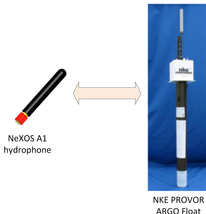
Figure 11 A1 hydrophone deployed on NKE PROVOR ARGO float
