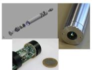
Compact, cost-efficient and integrated passive acoustic sensors. Improved transducer integration and processing will reduce size and cost while increasing functionality. Sensors are: A1 - low-power multifunctional hydrophone and A2 real time waveform streaming and pre-processing hydrophone array.
